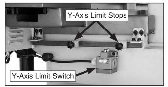
Figure 41. Y-axis limit switch and stops.
